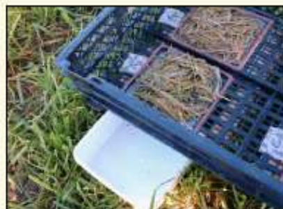
▲ Equipment for collecting leachate from green manure. In total 24 cells with 4.7 g DM in each, put out in the field on August 29.
